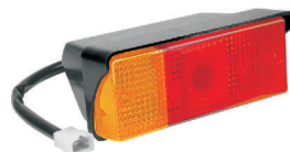
PAP-2714 Tail Lamp Assembly Suitable for: Surpanch/ 575 D.I. (N. Model) Spare Lens Part No. PAP-2761
